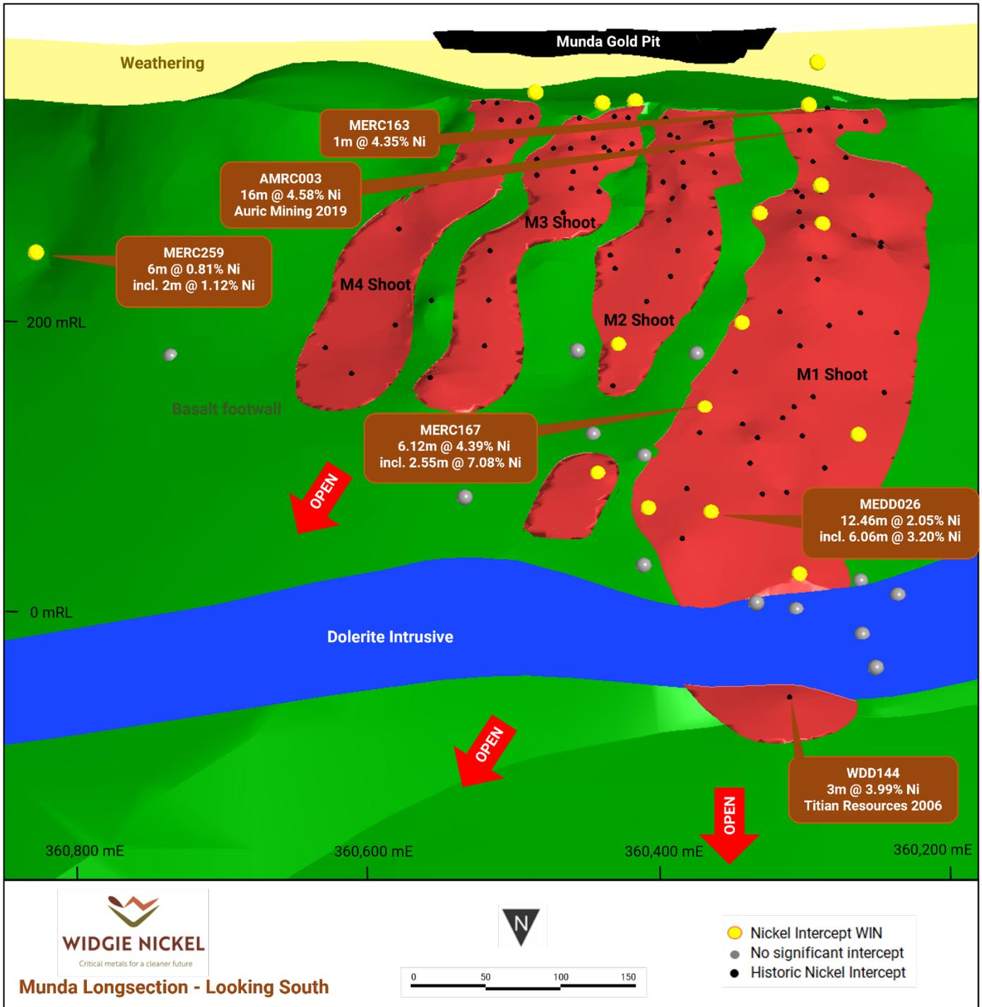
**Figure 1 – Munda longsection looking South – 2023 Geology interpretation with Widgie Nickel (WIN) and historic significant intercepts**
